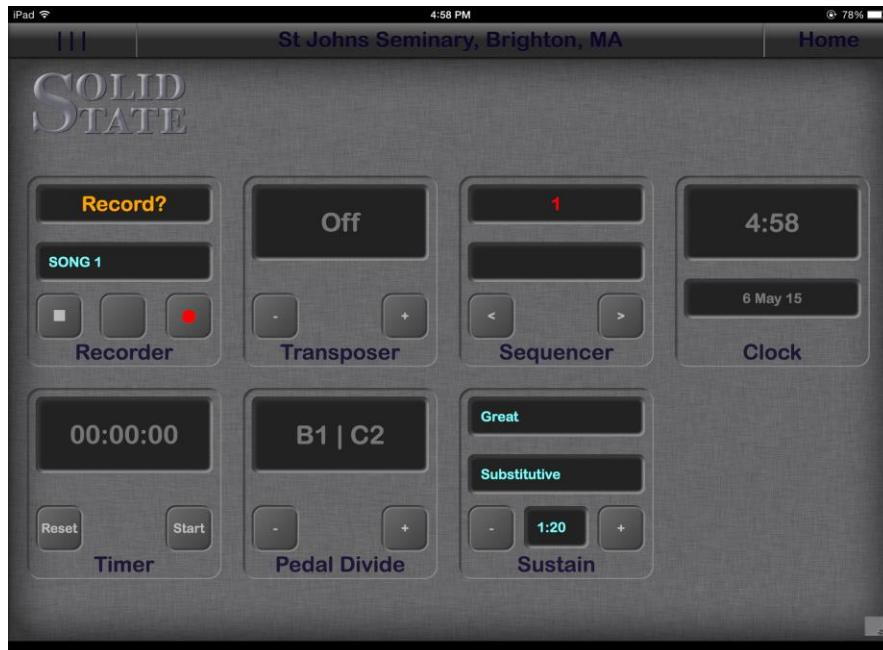
In this screenshot the recorder has been armed by pressing record once, to prevent accidental over recording of a previously recorded song it is necessary to press record again to start recording. Press stop to exit.
