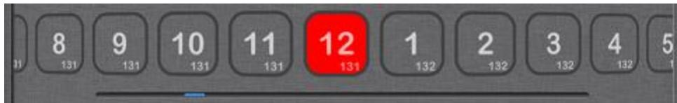
The Piston Selector carousel allows you to activate any piston in the sequence. Tap on the piston and the stops will move on the console. Spin the carousel left or right to access pistons that are not visible. There is a blue progress bar underneath to show you where you are in the sequence. As you play and press next the carousel will rotate keeping the current piston in view. Each piston shows both the piston number and the memory level.
