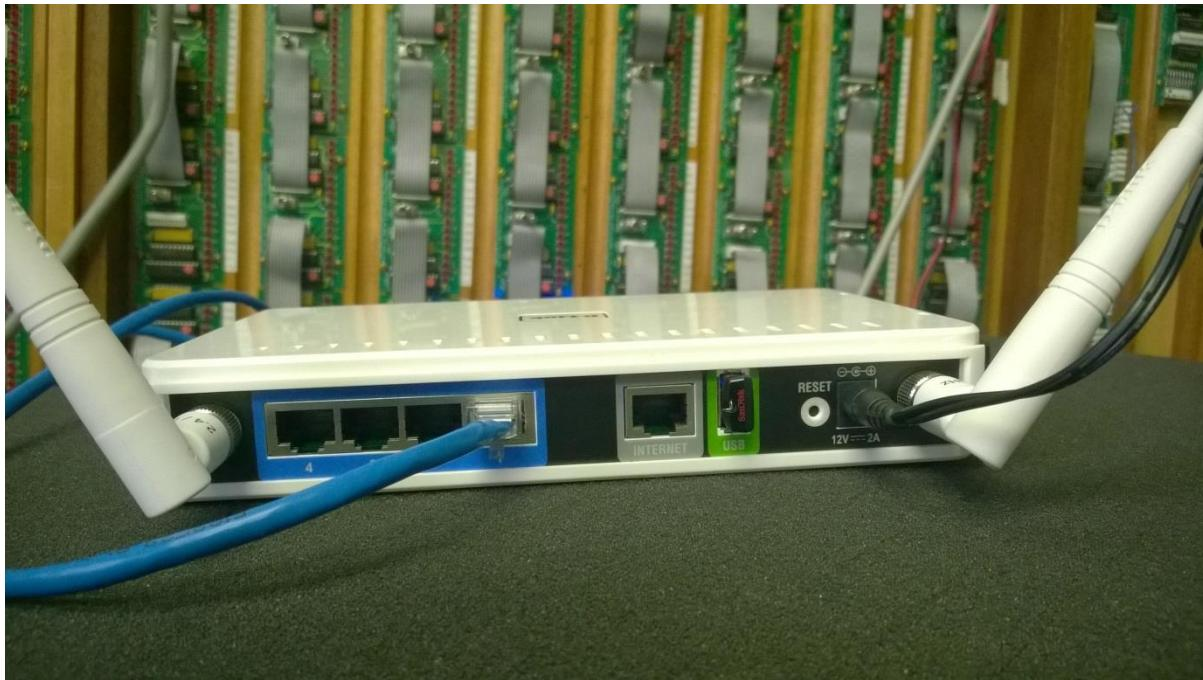
**POWER** - Connect the included power supply to the back of the MiniServer. The 1602 MiniServer can be powered permanently or with the organ. The MiniServer takes up to 2 minutes to start up and the Palette will not be available until the MiniServer has booted.
