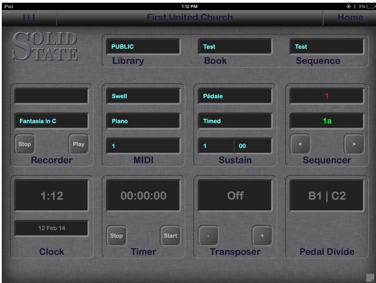
The Home Screen provides quick access to features through small panels called Modules. The choice of modules is defined by your organ builder to suit the design of the organ.
