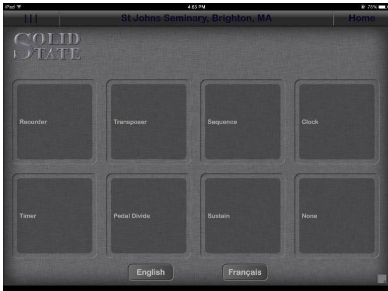
The Setup Screen allows you to choose the layout of the Modules on the [Home Screen](#).
