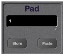
The Pad allows you to save piston settings for use in other parts of the Sequence.
