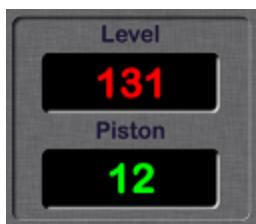
The memory display is a duplicate of the console display and shows the current memory level and the last piston that was used.
