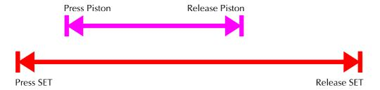
In normal operation the SET piston is pushed, held, and a divisional or General piston pushed. The stops drawn will then be stored.
