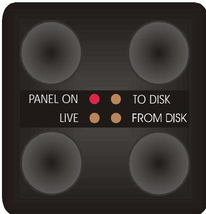
The complete Total Recall function is turned on and off using the PANEL ON button (top left). When the PANEL ON lamp is lit the other three buttons on the rest of the panel are operational.
