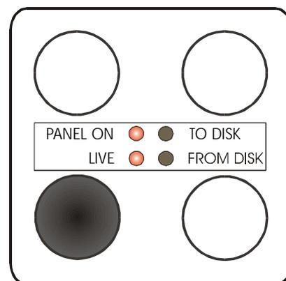
*To maintain the speed of response you are familiar with, the Total Recall System does not save the new settings to the floppy disk at this time but keeps them in its own memory until the LIVE button is pressed once more to exit. At this time, all registration settings within memory levels 1 to 32 are saved onto the disk. DO NOT remove the disk until the green light is off.*
