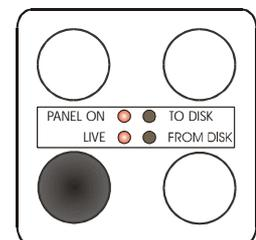
4/. When the LIVE lamp remains on with a steady glow the LIVE function is active and ready to use. Any pistons now set at the console within levels 1 to 32 will be recorded into Total Recall memory (not into the main MultiLevel Capture System memory).
