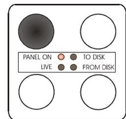
3/. Once the PANEL ON lamp is lit, push the LIVE button and hold in for three seconds until the disk can be heard being activated in the disk drive.
