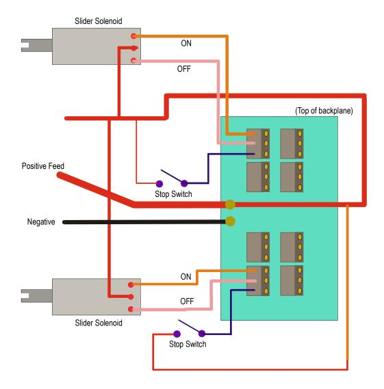
On the front of the card, close to the handle, are two adjustment controls for each channel. These control the ON and OFF power and are marked on the circuit board as X and Y. In the configuration above X controls the OFF power and Y controls the ON power. They can be adjusted with a small screwdriver.
