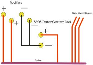
Make sure the order on the busbar is Power Supply - Direct Connect - Solenoids
