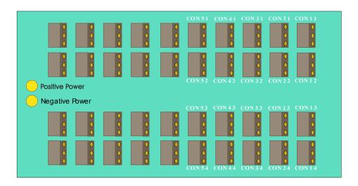
The exact number of terminals used will vary depending on which card type is installed. Please refer closely to the wiring information for each card type detailed in the following pages.
