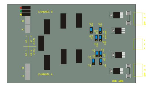
There are four jumpers grouped to the top of the card (Channel A) and an identical four to the bottom (Channel B). Each group of four jumpers will set the input polarity for one channel of the card.
