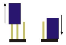
Once you have decided the required polarity, it can be a useful visual check to make sure all jumpers have the same pin exposed before inserting the card into the OB System Box.
