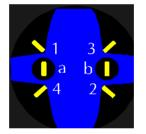
Lock-switch showing connections, use only pins 3 and 4.
