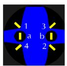
Lock-switch showing connections, use only pins 3 and 4.
