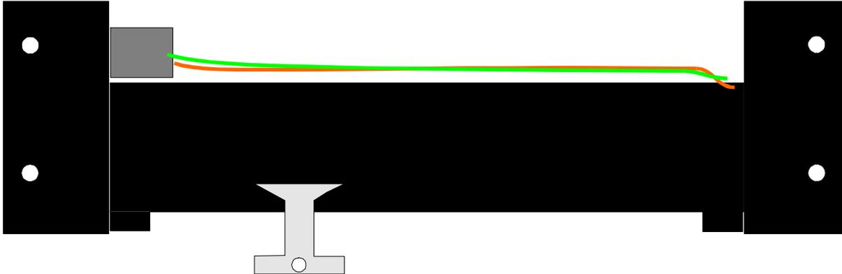
The moving arm on the encoder is connected to the crescendo pedal via a link that should be designed to prevent the organist forcing the encoder beyond its normal travel. The maximum travel is 104mm (4 1/8").
