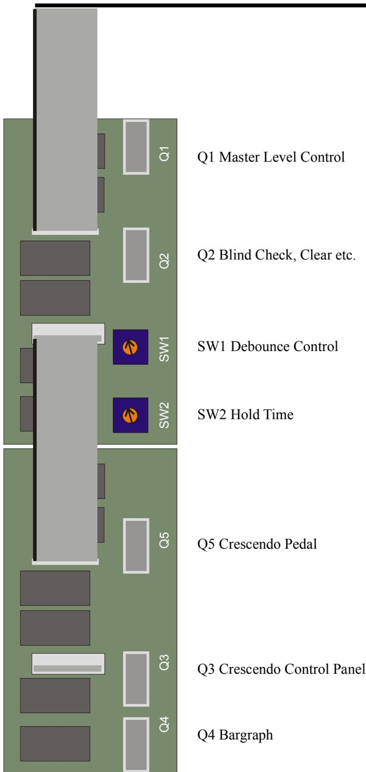
Each panel is connected to the console plane with a 10-way ribbon cable. The cables are supplied with the system in 6ft (2metre) lengths although longer cables are available to special order.
