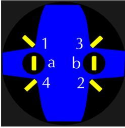
A rear view of the switch/lamp. The lamp connects to contacts 'a' and 'b'. Contacts marked 3 and 4 are normally open and should be used for the switch wiring.
